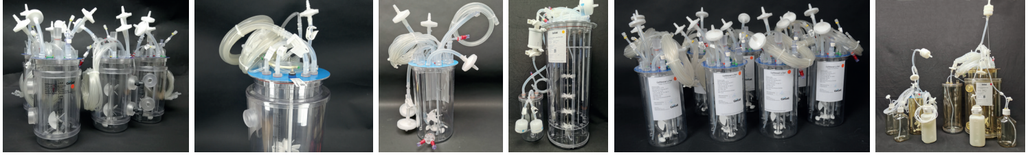
Above various SUBs and SUFs with thermal control by electrical blankets or liquid jackets. Media connections at bottom or head plate. Any impeller or turbine one can imagine.
