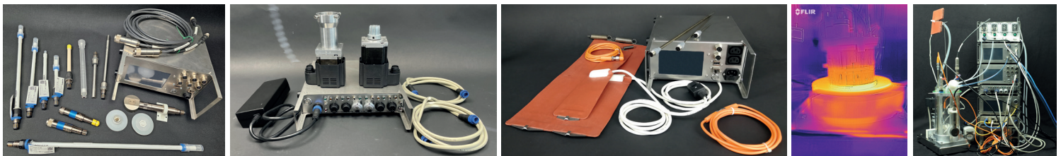
Process-Control-Systems (PCS) come from a range of suppliers. Most common is Sartorius, Applikon, Eppendorf and some 10 smaller manufacturers in Europe. All PCS based on operation principles originating from B.Braun (Melsungen, Germany) in the 70ties. Now typically ONE big box with input for temp, DO, pH and output for agitation, aeration and temperature. Are these PCS's customizable or easy to expand – NO.
