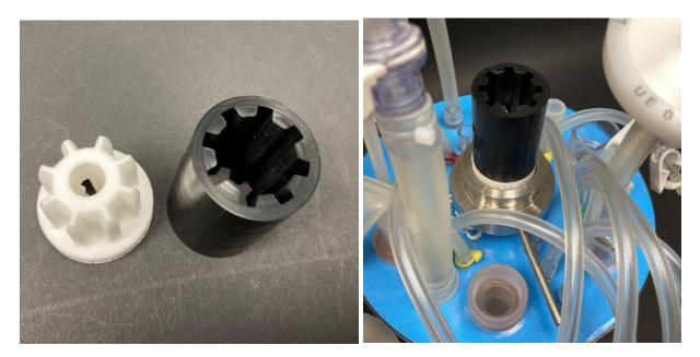
Mount the black rubber coupling onto the white sprocket ready for adding the servo motor.
