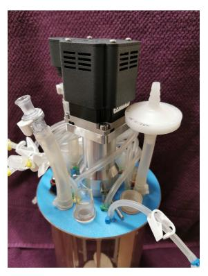
A range of drive systems for agitation mounted with the ID39-B servo motor adapters will now fit the CellVessel or BactoVessel.
