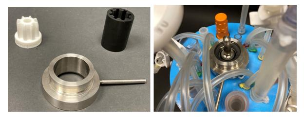
Photo show the white nylon sprocket, the smallest HPD-disc and the black rubber coupling. Photo to the right show a CellVessel OD 137 mm / 3.2 litre head plate mounted with the smallest ID39-B / HPD-disc on the HPD bearing.
