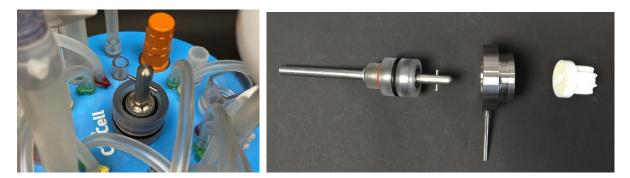
The centre HPD bearing is 30 mm in diameter and the drive axle is 8 mm in diameter. The 2 mm cross pin which pass through the 8 mm axle is designed to transfer rotational power from the white nylon sprocket to the agitation system inside the SUB, SUF, SUM.
