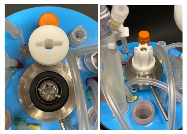
The HPD-disc is pressed gently onto / mounted on the HPD bearing body. Make sure, the HPD-disc do not squeeze any silicone tubes and is fitted tight towards the head plate. Hereafter the white nylon sprocket is mounted on the 8 mm axle. Ensure the slot in the white toothed sprocket fits over the 2 mm cross pin.
