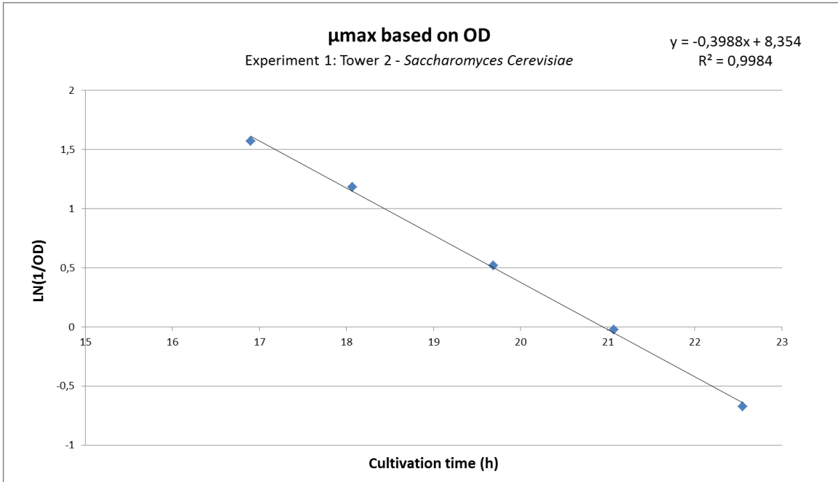
Figure 8: Determination of the maximum growth rate \mu_{max} based on OD measurements. OD measurements were only taken once which is the reason for no error bars
