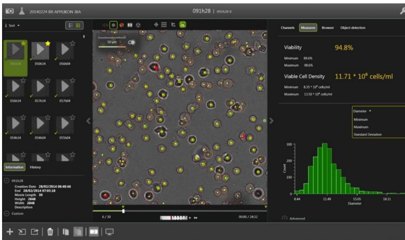
Figure 1: Screenshot of real-time monitoring of the cells. According to Ovizio the software is capable of distinguishing viable and dead cells based on light refraction. Viable cells will create a light cone, which will give a very high intensity light (lens effect), while dead cells will create a more scattered light. In this image viable cells are marked by green, and dead cells are marked by red. Whether or not a cell is classified as viable or dead is based on light scattering and cell diameter [6].
