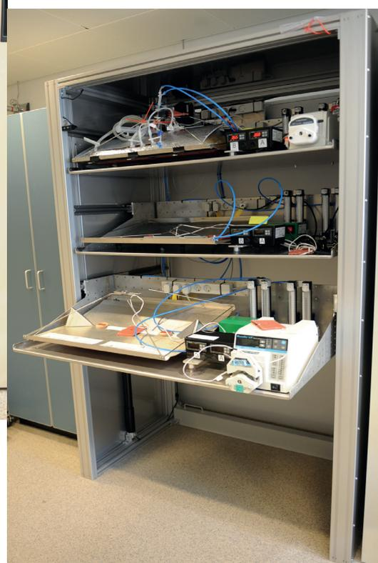
Ergonomic handling is important and requires traditional wave bag systems arranged horizontal on desktops next to each other. Not really efficient use of space! CerCell offer a cabinet with 3 shelf's each for one CellTumbler arranged vertical and operated with servo motors. Each shelf on bearings is easy to extract in the desired height for ergonomic handling.
