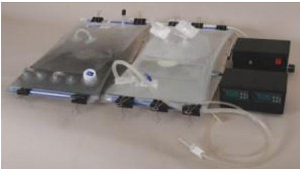
**Figure 3. CellTumbler platform.** CerCell's CellTumbler 2x5L fitted with Cell Bags (GE) used in the experiments.
