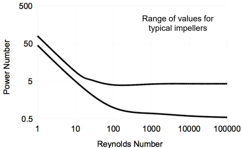
Power Number as a function of Reynolds number for a range of typical impellers.
