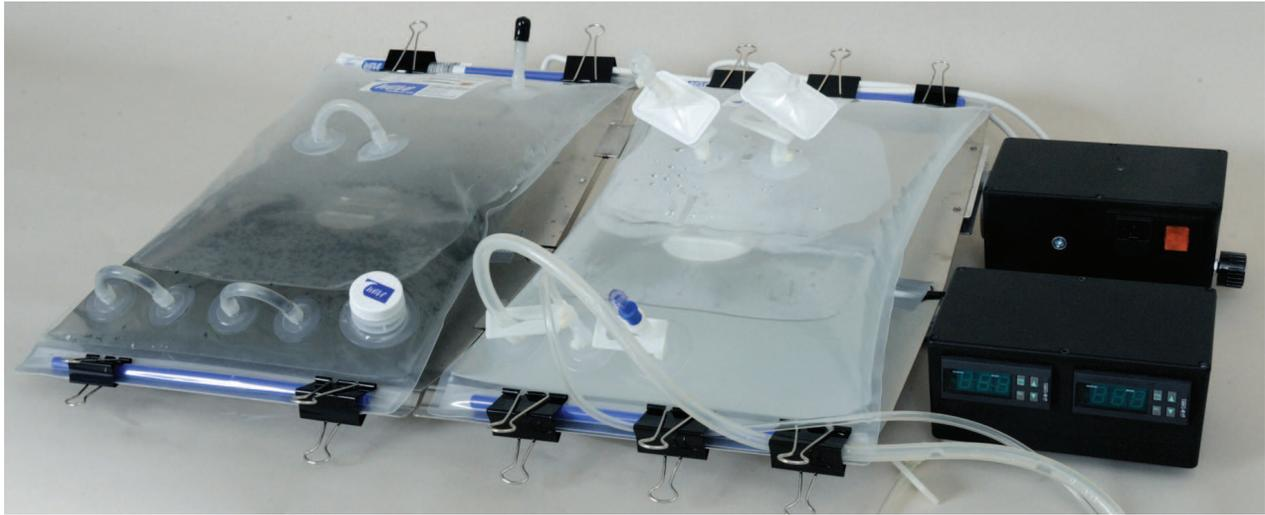
Any commercial available wave bag up to 10/20 litre may be used and operated independently with temperature and gas control.
