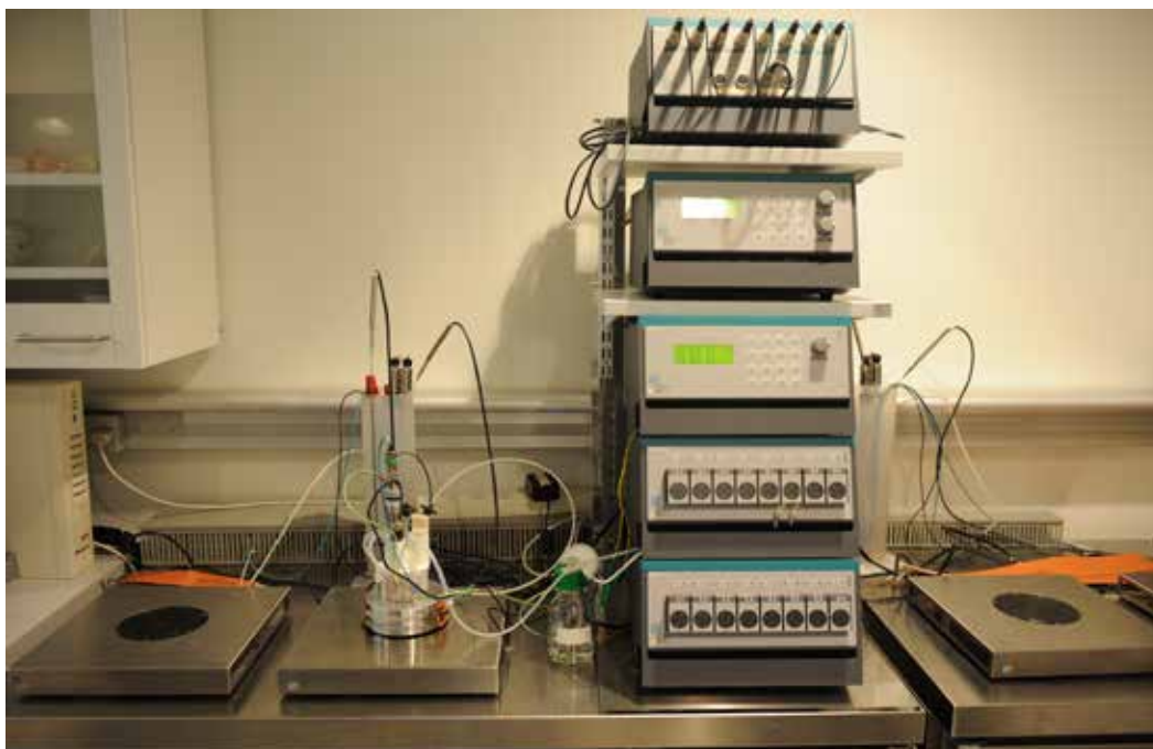
Smallest CellVessel 23-0250 on well known DasGip MP8 PCS and M10 MST (60-1500 rpm) for mammalian and stem cell cultivation. The aluminum Heating-Support-Foot (HSF) insure mechanical support of the tiny and low thermal mass CellVessel 23-0250 STR and facilitates stable thermal control by the PID of the PCS.
