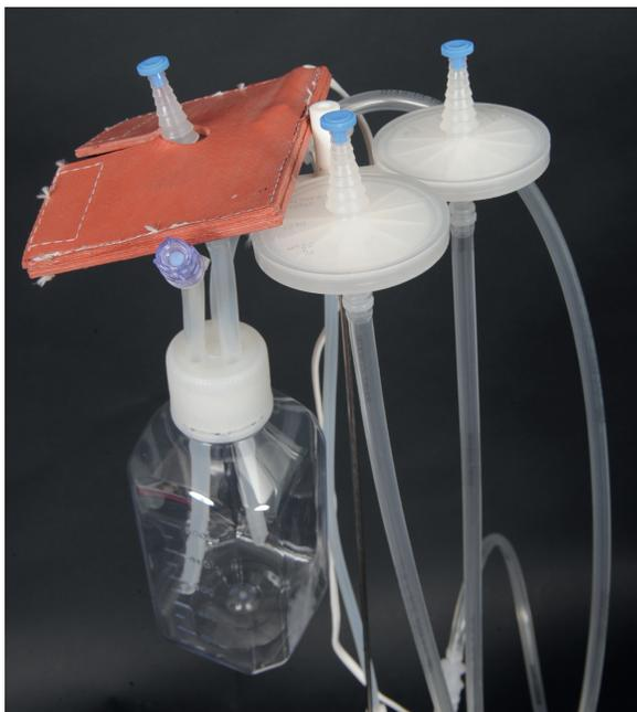
BactoVessel 25 series of Single-Use-Fermenter (SUF) for microbial fermentation facilitates a range of accessories such as single-use exhaust gas cooler, filter heater, bubble traps, etc. Here a used p/n 25-5000 is shown including gas cooler and dual exhaust filters.
