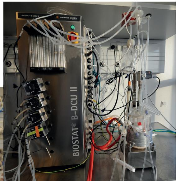
Biostat with water heating in perfusion setup controlling a CellTank for one month cultivation of CHO suspension cell line. Bio mass sensor amplifier is visible.
