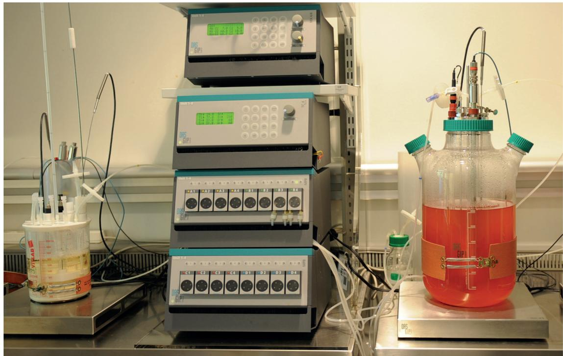
Work at Bioneer in Denmark on CellTank in perfusion on DasGip MP8 with identical suspension CHO cell lines compared to autoclaved 8 litre glass STR. Both STR and SUB hold  $1.5 \times 10^{10}$  cells. The SUB operates for weeks or month in perfusion setup. The traditional STR with 6 litre wv was cultivated for 6 days before termination due to extensive lactate levels.
