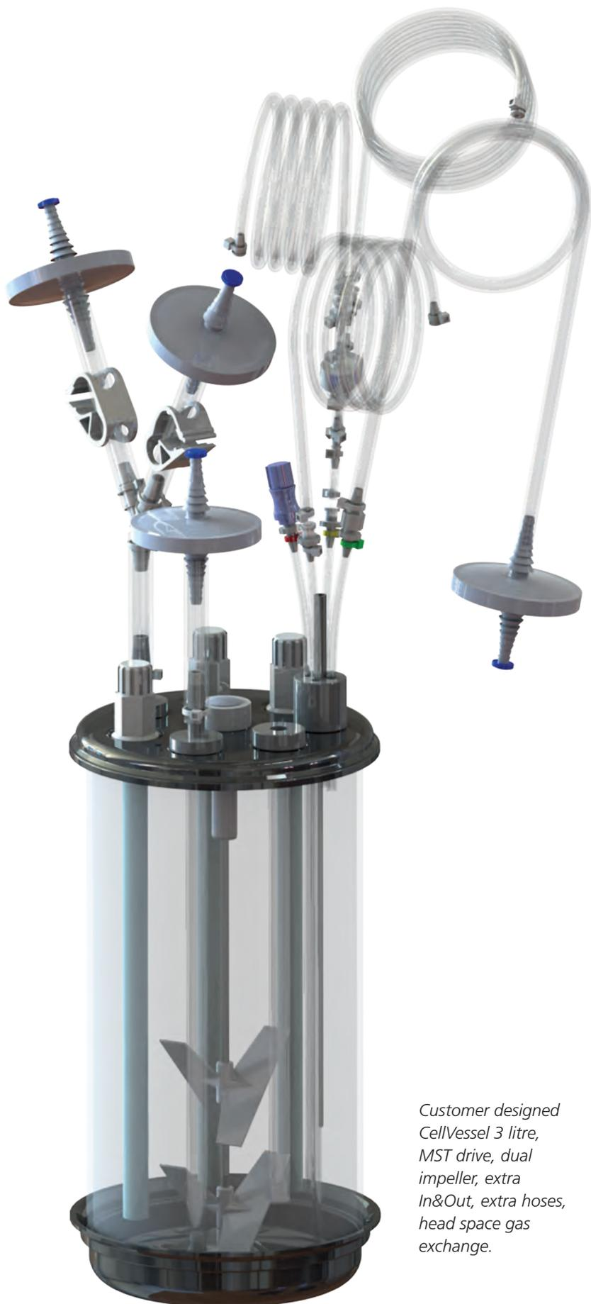
*Customer designed CellVessel 3 litre, MST drive, dual impeller, extra In&Out, extra hoses, head space gas exchange.*
