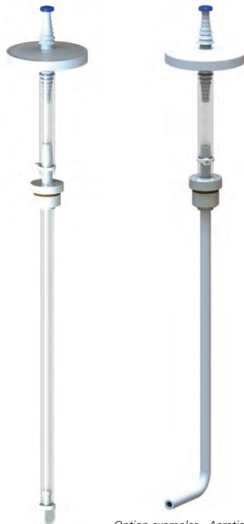
*Option examples - Aeration devices, Micro – PP body with 15 µm pore, Macro – multiple 500 µm holes in tube, L-sparger with 10 x 0.3 mm holes in OD8 mm tube.*
