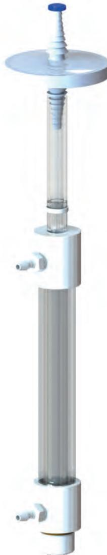
Option example - 4 ports with female Luer-Lok = one sample line with swabable valves 40 mm above bottom, one harvest line to vessel bottom, two headspace lines, ground SS probe integrated
