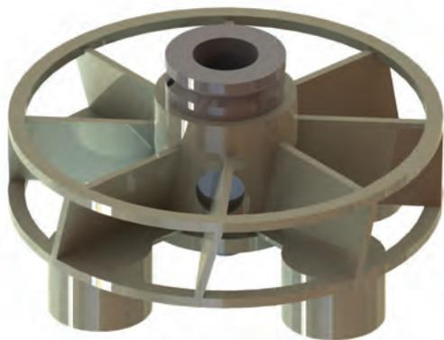
OD80 mm turbine integrating porous PP sparger bodies in the core, 4 magnets for MST drive at 1500 rpm
