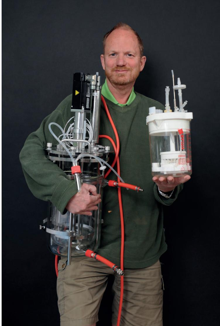
*Light weight rigid plastics CellTank compared with 5 litre jacketed glass/steel STR. Equal total cell density and daily product expression though CellTank offer 4-8 times the cultivation time.*
