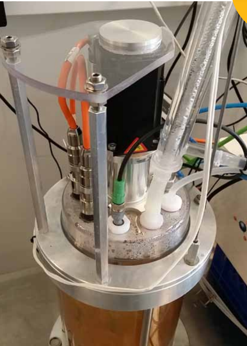
BactoVessel 5.7 litre facilitating Smith turbine and Marine impeller operating at 1,500 RPM mounted in Re-Usable-Jacket, RUJ equipped with servo motor support and Sky-Support for the gas-cooler and exhaust filter.
