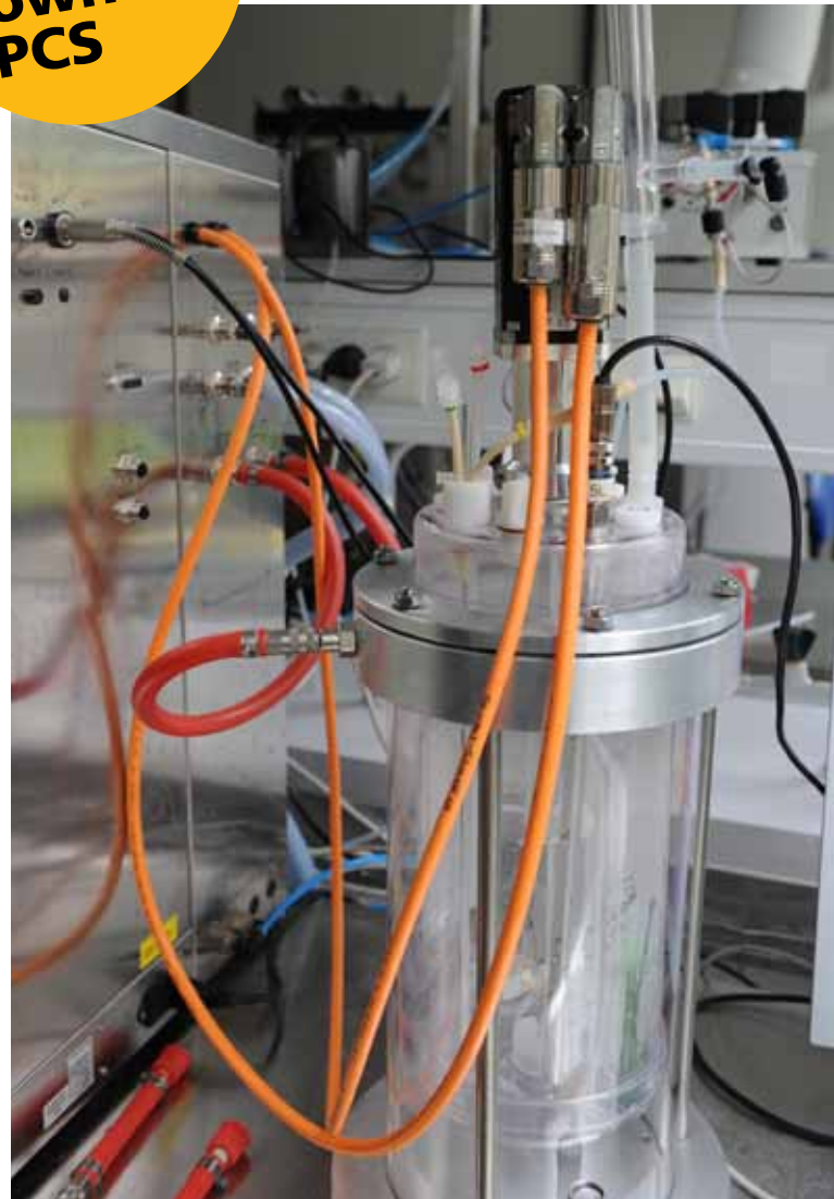
Kollmorgen AKM23D servo motor driving via HPD in Biostat setup a 5.7 litre BactoVessel submerged in a RUJ
