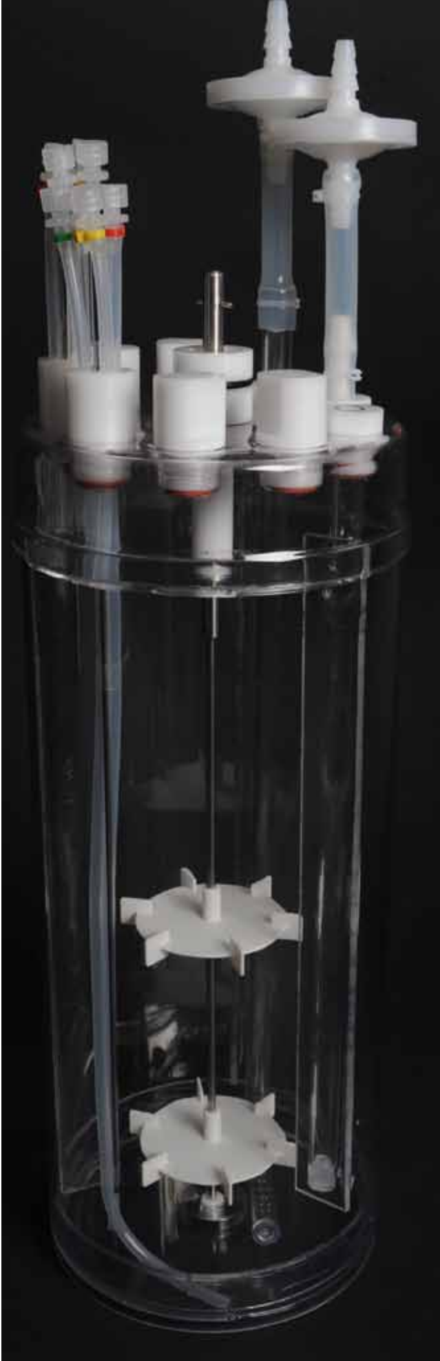
OD130 x 420 mm BactoVessel customised to end-user requirement integrating 3 baffles, ring sparger, dual In&Out, HPD drive and two specific Rushton turbines.
