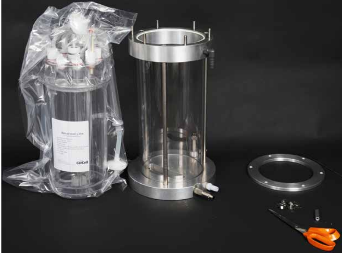
Customised 5.7 litre SUB for Head-Plate-Drive next to the Re-Usable-Jacket for heating prior the installation.
