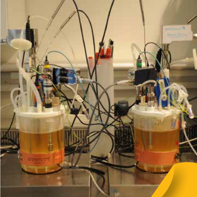
Two identical 2 litre SUB on Magnetic-Stirrer-Tables equipped with 50x380 mm silicone heating blanket. Power rated at 110 watt from 230 VAC supply.
