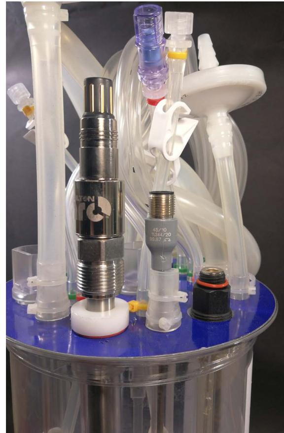
The complete **CellVessel SUB family** optional may include through the head-plate vertically mounted, pre-installed Single-Use-Sensor's (SUS) for DO, pH, °C, and level.
