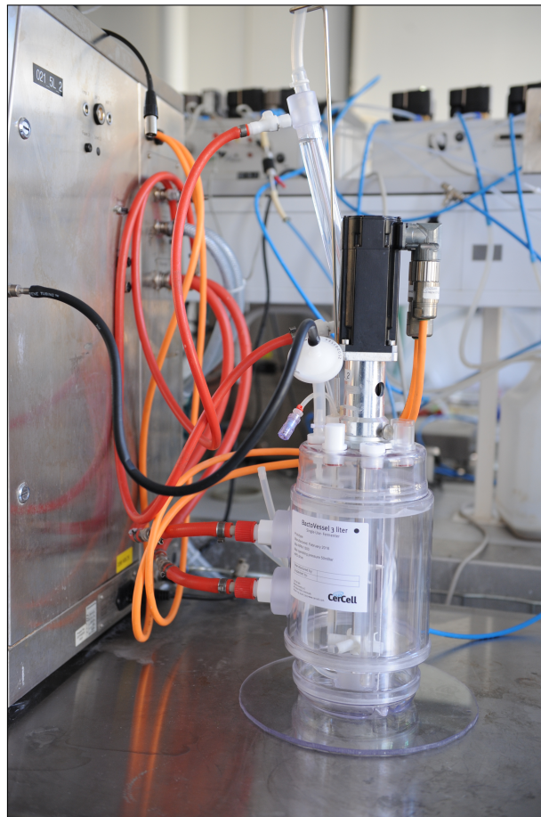
Figure 7: The fermentations carried out for the experiments upon this project were done with this 3 liter single-use fermenter prototype from CerCell ApS.
