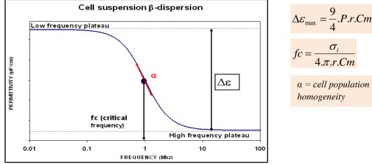
*P* = Biovolume (volume fraction ; r = cell radius ; Cm = membrane capacitance ; σi = intracellular conductivity
