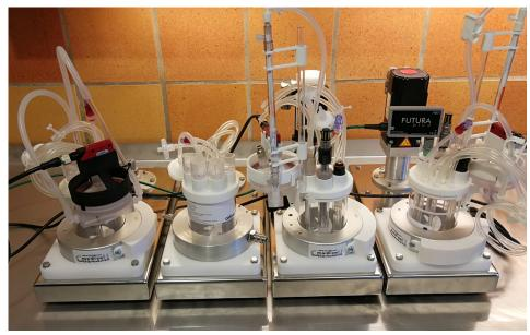
These 4 in parallel operating MST can handle 500 ml VV as well as 3,200 ml VV SUB's or PR-SUB's in only 80 cm table space controled by any PCS you may have.
