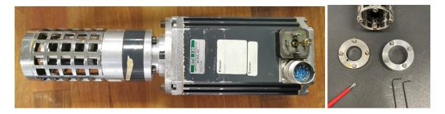
The CerCell kit consist of a metal replacement adapter incl 4 Allan bolts. The original front coupling has internal conical design fitting the B.Braun / Biostat combined stainless steel / glass bioreactor head plate from the 80ties. The CerCell replacement has internal cylindrical ID39 mm hole which fit to all the ID39-B format couplings.
