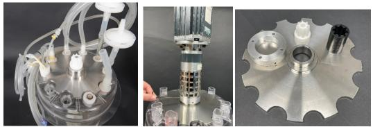
Easy mounting on CerCell MST as well as on the OD250 mm CellVessel or OD250 mm BactoVessel HPD drive. Center photo show how you with al Allan key secure the two metal parts from the kit. Photo at right show the complete kit for Heidorph conversion.
