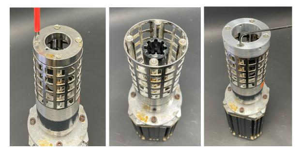
Remove the 4 standard M4 screws and mount the new adaptor with 4 new Allan screws.
