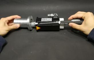
The metal sprocket inner hole dimension depends on the particular servo motor shaft size.
