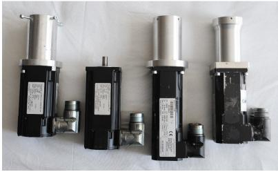
One Kollmorgen AKM servo motor with standard Biostat ID39-B adaptor mounted on the CerCell MST. A set of Kollmorgen servo motors with almost identical size (metric or inch) adaptors and one shaft.
