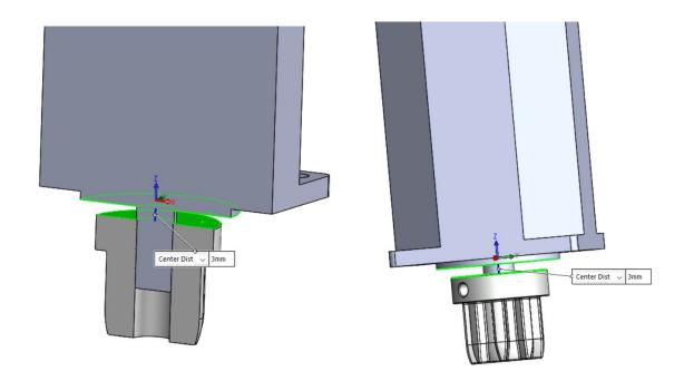
Rendered sketches of the motor mounted with the metal sprocket. Distance between motor flange and sprocket app 2-3 mm or app 1/8".
