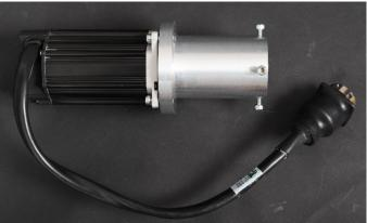
CerCell seek to use bolts with internal hexagonal sockets. The Allen keys are metric and of M4 size or M5 bolt for connecting motor and adapter via nuts. The 4 bolts should be tightened with max 1-2 Nm or 1-2 lbf/feet torque.
