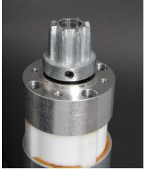
CerCell seek to use bolts with internal hexagonal sockets. The one M8 bolt should be tighten 2-3 Nm or 2-3 lbf/feet torque.
