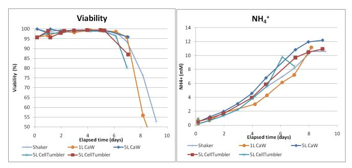
**Figure 2. Viability and ammonium.** Viability curves are very similar in all systems (left).  $NH_4^+$  (right) measured by BioProfile.
