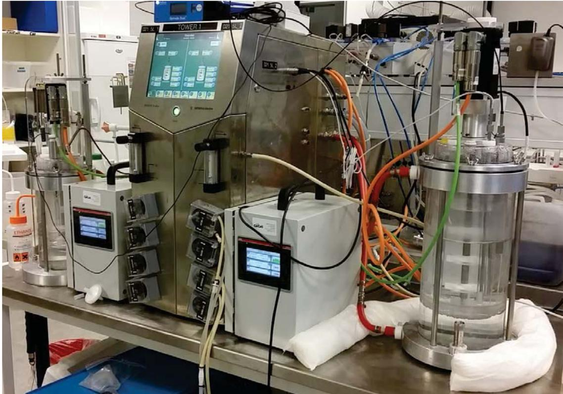
*STR left against SUF right comparison both liquid cooled and connected to the twin channel Biostat PCS with liquid thermal control. SUF installed in a Re-Usable-Jacket for efficient heat transfer. Two independent servo motor drives in order to reach the 2000 RPM target. Photo by Per Stobbe.*
