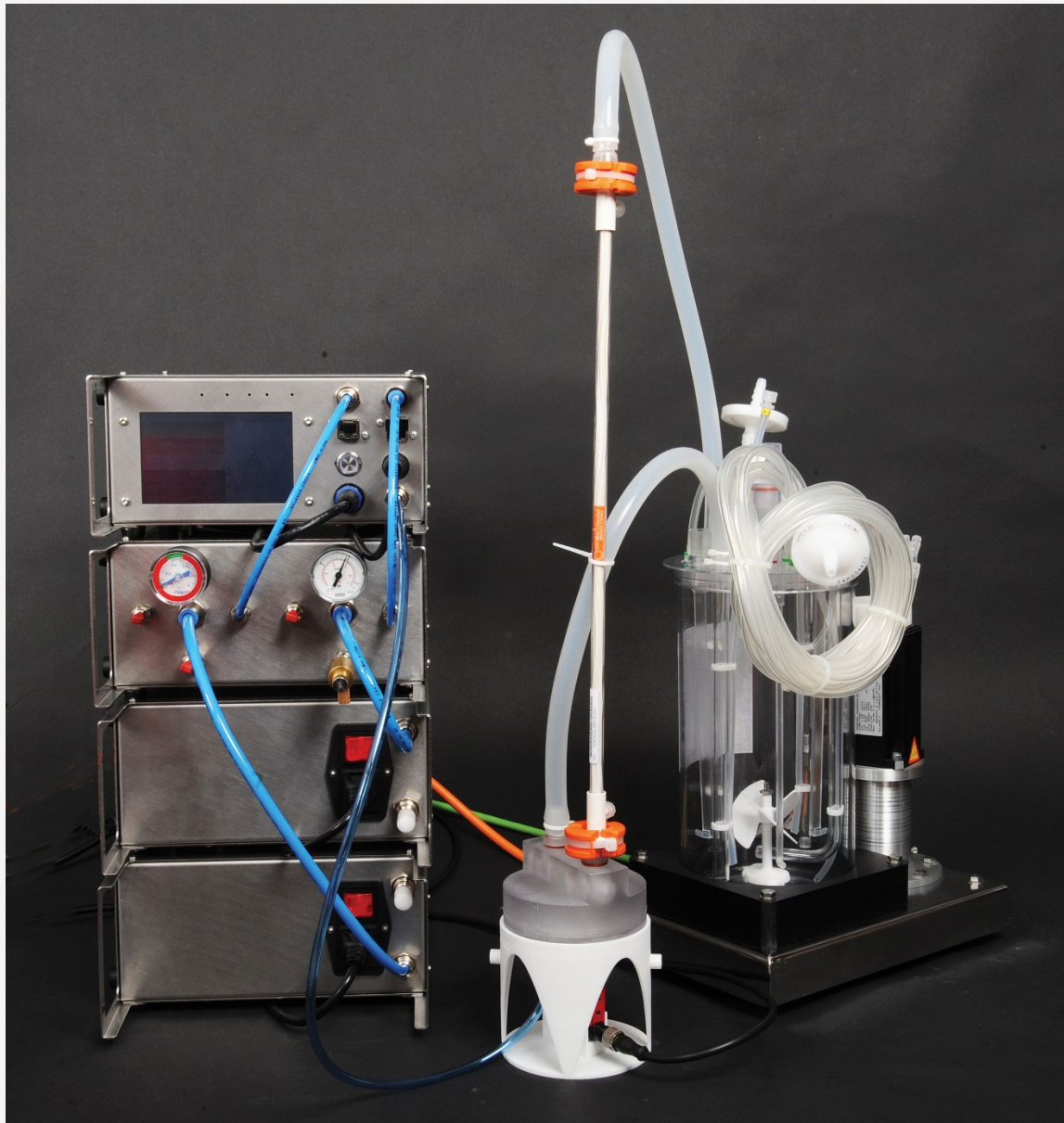
Figure 2. PerfuseCell asserts that its CellMembra system qualifies as a single-use, scalable bio-reactor for adherent cell culture.
