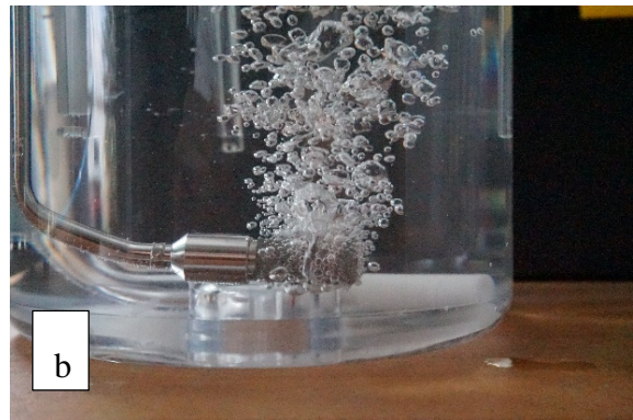
Figure 17. Comparison of the straight tube with a plastic sparger attached on it (a.) no modification in the design and (b.) metallic sparger on L-shaped tube flow rate location: 60cm.
