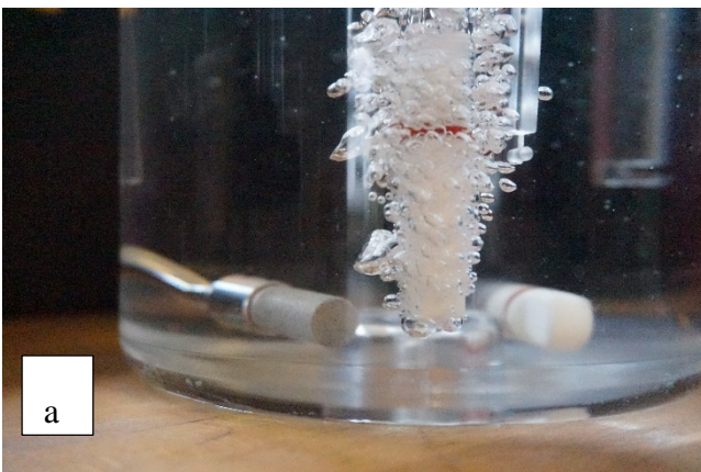
Figure 26. Comparison of the straight tube with a plastic sparger attached on it a. no modification in the design, b. sparger glued on the tube. Flow rate location: 60cm.
