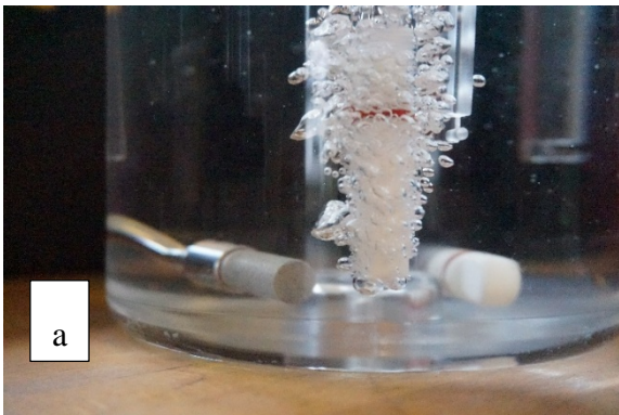
Figure 17. Comparison of the straight tube with a plastic sparger attached on it (a.) no modification in the design and (b.) metallic sparger on L-shaped tube flow rate location: 60cm.
