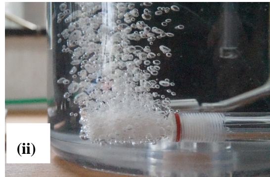
Figure 9. Bubbles generation through different spargers at air inlet flowrate 62.98 ccm. (i) metallic sparger, (ii) cylindrical single use sparger, (iii) porous disk X2, (iv) porous disk X3, (v) porous disk X2 in sparger body for two, and (vi) porous disk X2 in sparger body for three.
