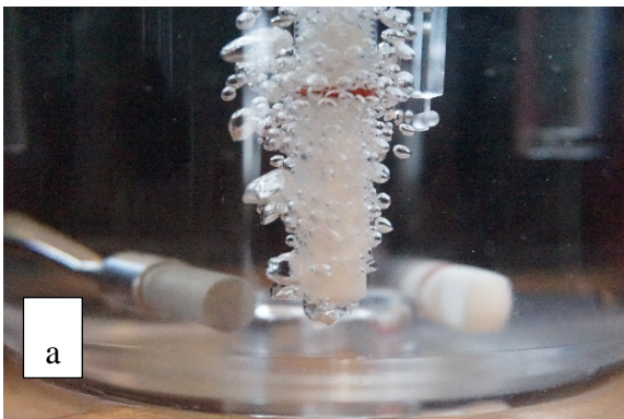
Figure 16 Comparison of the straight tube with a plastic sparger attached on it (a.) no modification in the design and (b.) metallic sparger on L-shaped tube flow rate location 20cm.
