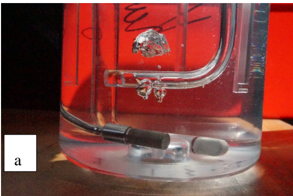
Figure 21. Bubble generation. (a) two orifices and (b) three orifices. Flowrate: 30mm (ball location).
