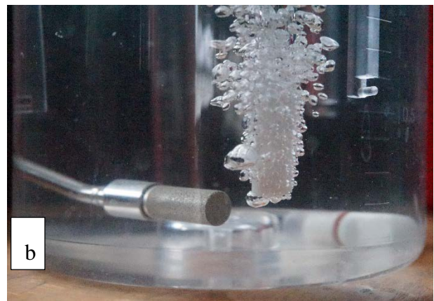
Figure 26. Comparison of the straight tube with a plastic sparger attached on it a. no modification in the design, b. sparger glued on the tube. Flow rate location: 60cm.
