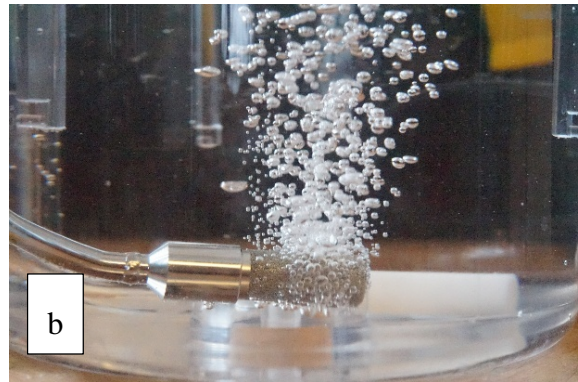
Figure 15. Comparison of the straight tube with a plastic sparger attached on it (a.) no modification in the design and (b.) metallic sparger on L-shaped tube flow rate location 20cm.
