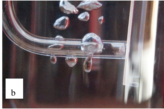
Figure 20. Bubble generation. (a) two orifices and (b) three orifices. Flowrate: 20mm (ball location).
