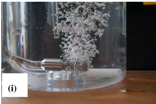
Figure 8. Bubbles generation through different spargers at air inlet flowrate 49.98 ccm. (i) metallic sparger, (ii) cylindrical single use sparger, (iii) porous disk X2, (iv) porous disk X3, (v) porous disk X2 in sparger body for two, and (vi) porous disk X2 in sparger body for three.
