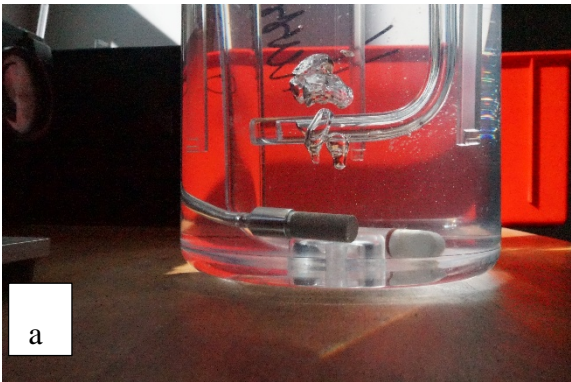
Figure 22. Bubble generation. (a) two orifices and (b) three orifices. Flowrate: 40mm (ball location).
