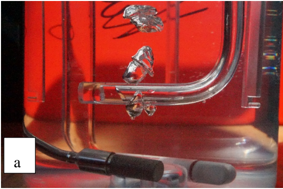
Figure 20. Bubble generation. (a) two orifices and (b) three orifices. Flowrate: 20mm (ball location).
