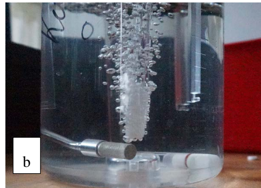
Figure 25 Comparison of the straight tube with a plastic sparger attached on it (a. no modification in the design, b. sparger glued on the tube). Flow rate location: 40cm.
