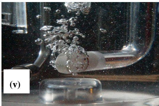
Figure 10. Bubbles generation through different spargers at air inlet flowrate 78.20 ccm. (i) metallic sparger, (ii) cylindrical single use sparger, (iii) porous disk X2, (iv) porous disk X3, (v) porous disk X2 in sparger body for two, and (vi) porous disk X2 in sparger body for three.
