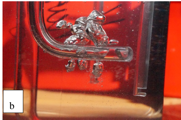
Figure 22. Bubble generation. (a) two orifices and (b) three orifices. Flowrate: 40mm (ball location).
